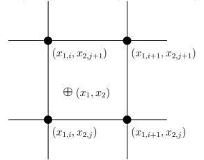
This bracketing can be done by bracketing in the two dimensions one at at time, using the technique discussed earlier.
